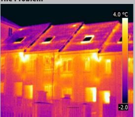
This image highlights the areas of heat loss in a row of terraced houses. Of particular note is the heat loss at the top of the junction where the party wall cavity meets the external cavity. ARC's T-Barrier will reduce heat loss along the edges of the party wall.
