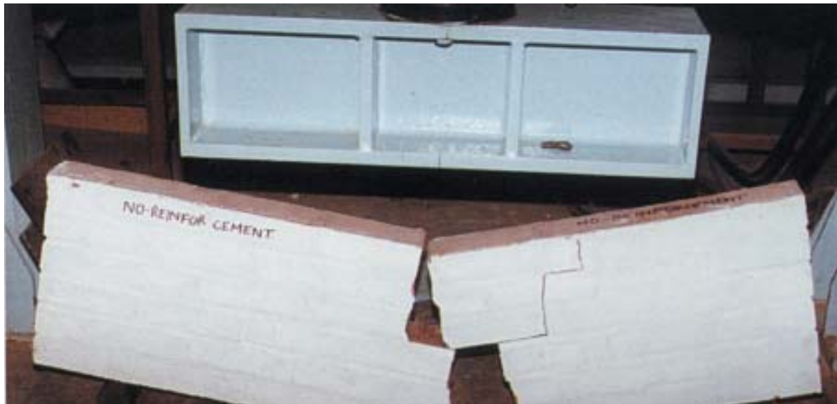
Destruction testing of un-reinforced wall
