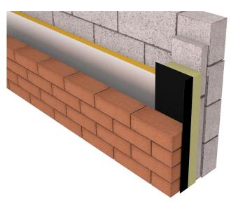
The ARC Rockfibre Insulated DPC has been developed to close masonry cavities for thermal, acoustic and fire applications. The primary reason for fitting the ARC Insulated DPC is to close off cavities around window and doors preventing cold bridging. Can easily be installed as the brick and block work progresses where a traditional block return is used.
